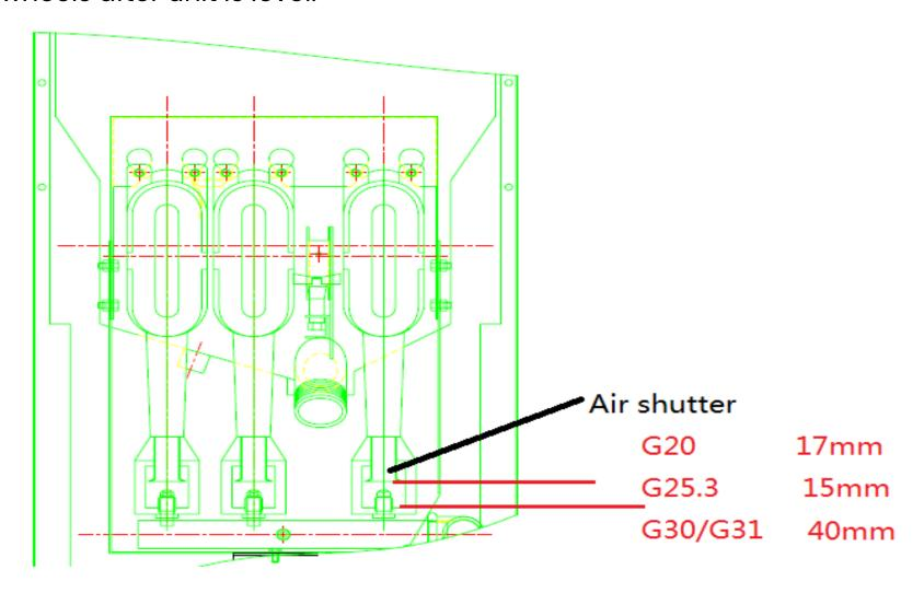
Unscrew the locking screw of the burner air shutter and adjust the air shutter to desired height. In the above picture, you can find the suggested height for different types of gases. The height is the distance between burner base and air shutter.
