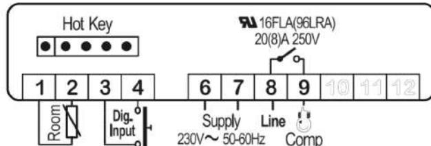
NOTE: The compressor relay is 20(8)A or 8(3)A depending on the model.
