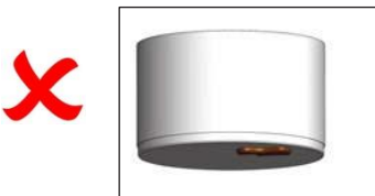
Figure 14 Excessive food spillage stuck to pan base will impinge the pan balance. One side of the utensil will be further away from the induction field than the other. This could reduce efficiency and it will also cook one side of the pan faster. Keep pans clean to ensure efficient cooking.
