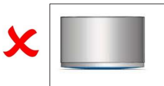
Figure 12 Pan base is bowed out and is NOT FLAT . The unit efficiency will be dramatically reduced during cooking. It may not even be detected by the appliance. Note: This is also liable to happen if pans are damaged, e.g. large dents.
