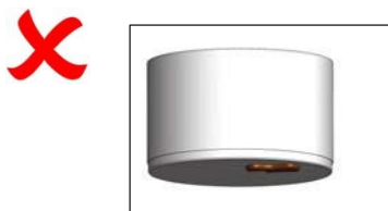
Figure 16 Excessive food spillage stuck to pan base will impinge the balance the pan. One side of utensil will be further away from induction field than the other. This could reduce efficiency and also cook one side of the pan faster. Keep pans clean to ensure efficient cooking.
