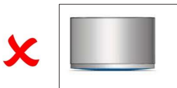
Figure 14 Pan base is bowed out and is NOT FLAT. The unit efficiency will be dramatically reduced during cooking. It may not even be detected by the appliance. Note: This is also liable to happen if pans are damaged, e.g. large dents.
