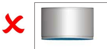
Figure 15 Pot base is bowed inward and is NOT FLAT; The unit efficiency will be dramatically reduced during cooking. It may not even be detected by the appliance. Note: This is also liable to happen if pans are damaged, e.g. large dents.
