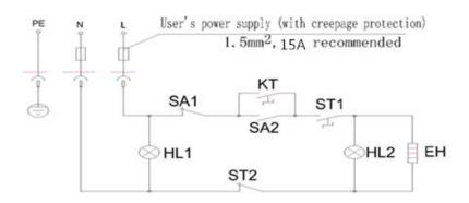
SA1:Power Switch SA2:Safe Switch ST1:Temperature Controller ST2:Limit Temperature **HL1:Power Indicator HL2:Heating Indicator**
