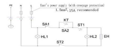
SA1:Power Switch S. ST2:Limit Temperature EH: Heating Element I
