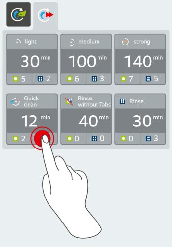
Quick cleaning easily found and quickly activated: simply place the cleaner tabs in the floor drain strainer and start the clean. Production can then resume after no more than 12 minutes.
