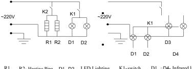
R1 、R2- Heating Pipe D1 D2- LED Lighting K1-switch D1 -D4- Infrared lamp K1 switch K2 Thermostat
