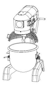
Note: When the cage assembly is in the closed position, a stop will prevent it from rotating in an anticlockwise direction.
