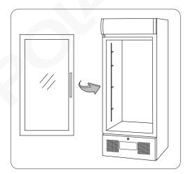
6. Disassemble the right upper hinge.
