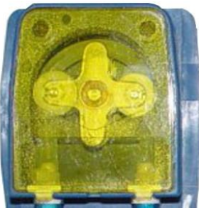
Example image of dosing equipment with peristaltic tube
